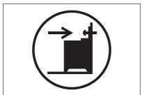
Install the anti-tilt protection 232 -237 mm down from the top surface of the appliance and 110 - 115 mm from the side of the appliance into the circular hole on a bracket. Screw it into the solid material or use applicable reinforcement (wall).
